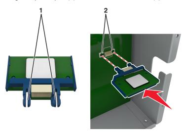
**4** Push the card firmly into place as shown in the illustration.
